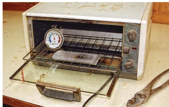
Toast. Temper in toaster oven for one hour at 350° F. This restores necessary toughness to the tool steel while resulting in Rockwell 62C hardness.
