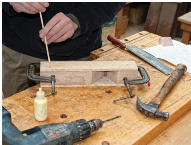
Dowel both sides. Two 3/16" pins on both sides will prevent movement under pressure. While two clamps hold the core blocks to the alignment board, drill 1/2"-deep holes for the pins, which are then cut off flush. Final clamping can be done in the bench vise like the 12"-wide one in the background here, or with clamps.
