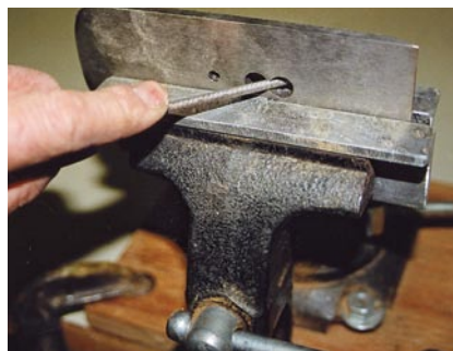
Blade beginnings. Making the blade begins with a 3/8" slot and hole for the rest button. The 25° angle is ground and the top rounded.
