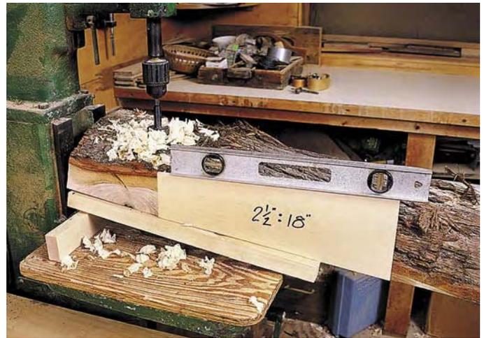
To achieve the desired leg splay, use a level on top of a board cut to the ratio of  $2\frac{1}{2}$ " to 18". This is the angle both end-to-end and side-to-side. The heavy slab rests on wood blocks to steady the drilling with a  $1\frac{3}{4}$ " Forstner bit in the drill press.
