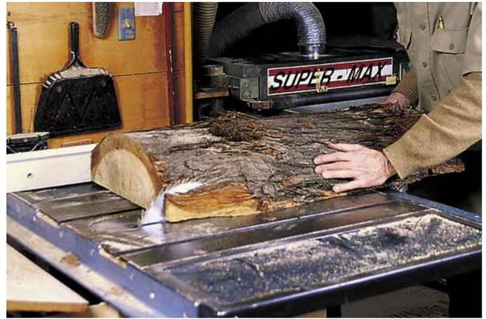
Trimming the top to size can involve a variety of tools: table saw, circular saw or chain saw. Leave an edge about  $1\frac{1}{2}$ " wide.
