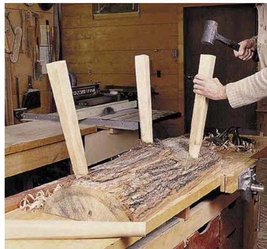
Hammer the legs into place. With this version of the garden bench with stopped holes, no glue or wedges are necessary, as the legs, being drier than the slab top, will hold tight as the top dries.
