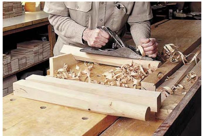
Prepare the legs using a V-notched board and a stop block. Plane the 2" x 20" squares so the bottom remains square and the top end is octagonal.
