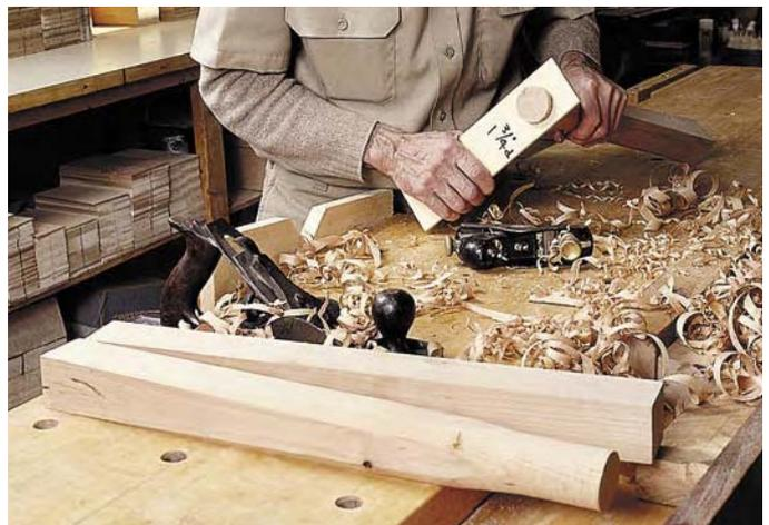
If you don't own a rounder plane, you can use a block plane to form the tenon. Whichever method you choose, use a hole gauge to check the tenon's size.
