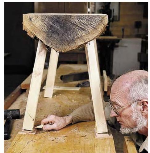
The final leg length is marked by leveling the bench (note the use of wood scrap under each shorter leg) and marking with a scribe. Cut along the lines and plane all sharp edges as the final step.
