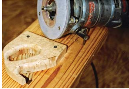
Handle. The handle is cut out and routed for curves. The two screws holding the handle for this operation are in the bottom edge that will be cut off.
