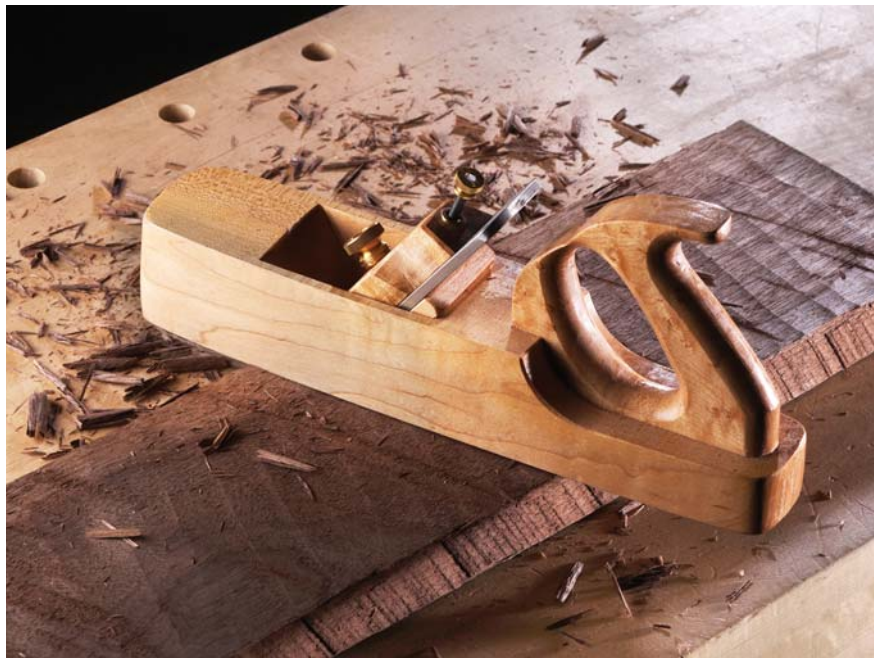
Jack of all trades. Jack planes can be used for both roughing and smoothing chores. This shop-made example allows you to change the pitch of the iron. Low for rough work. High for fine.
