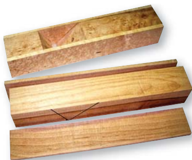
Three-piece body. By dividing the plane box into three pieces, the angles of the blade pocket can be easily and accurately made: a 45° bedding angle, a 60° front angle and one small 90° cut in the front block.
