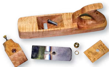
Makeup. The elements of a jack plane with double-screw adjustment: Razee plane body, cap with holding and adjustment screws, blade with rest button, and 52° wedge for optional smoothing plane pitch.
