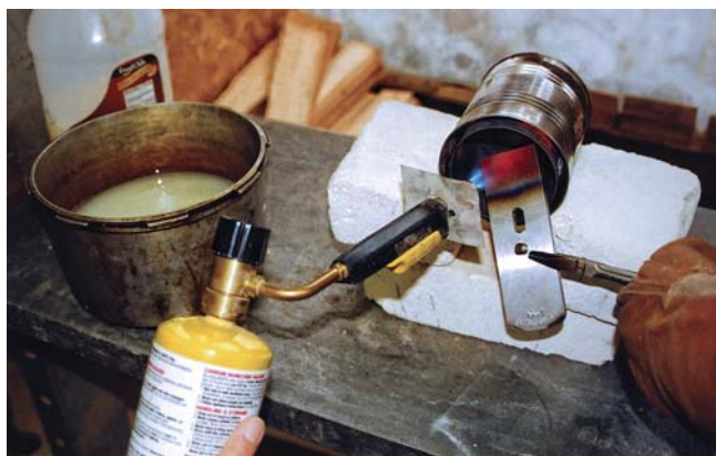
Homemade furnace. Harden the cutter using a torch and furnace made of nested tin cans. Quench when red hot. A 2" x 2" piece of sheet metal with a hole (slid over the end of the torch) protects the plastic from heat.
