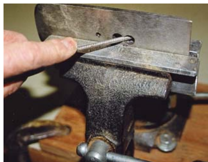
Blade beginnings. Making the blade begins with a \frac{3}{8} " slot and hole for the rest button. The 25^\circ angle is ground and the top rounded.
