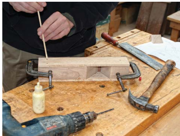
Dowel both sides. Two 3/16" pins on both sides will prevent movement under pressure. While two clamps hold the core blocks to the alignment board, drill 1/2"-deep holes for the pins, which are then cut off flush. Final clamping can be done in the bench vise like the 12"-wide one in the background here, or with clamps.
