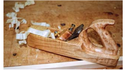
Fine-tuning. Sharpen the blade, make the blade square to sole and adjust the cap.
