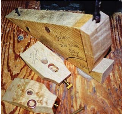
Two-screw mechanism. Drilling the top screw at 15° will hold the inverted thumb nut. The back of the cap has space for the rest button and a 3/8" lead screw hole. The front of the cap has wear washer and adjustment rod.
