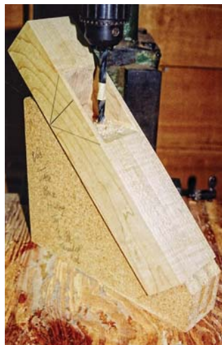
Drill for 3/8" threaded rod. Use of a jig helps hold the plane body at 45°. A pre-drilled 3/16" hole keeps the 2 1/64" drill on line.
