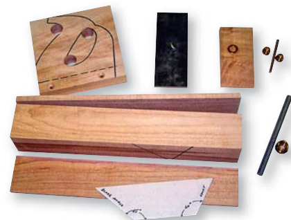
Parts. Parts of the jack plane: Handle with 3/4" holes prior to cutting, blade, cap parts, core block and sides, angle pattern, lead screw and thumb nut.
