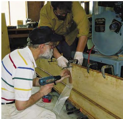
In a 12'-long boat, the plywood must be scarf jointed for length. The long beveled overlap joint uses scrap blocks on each side squeezed together with deck screws. Merlin (left) and Rick Eisenlord use waxed paper to prevent the blocks from being epoxied to the hull, as you see here.
