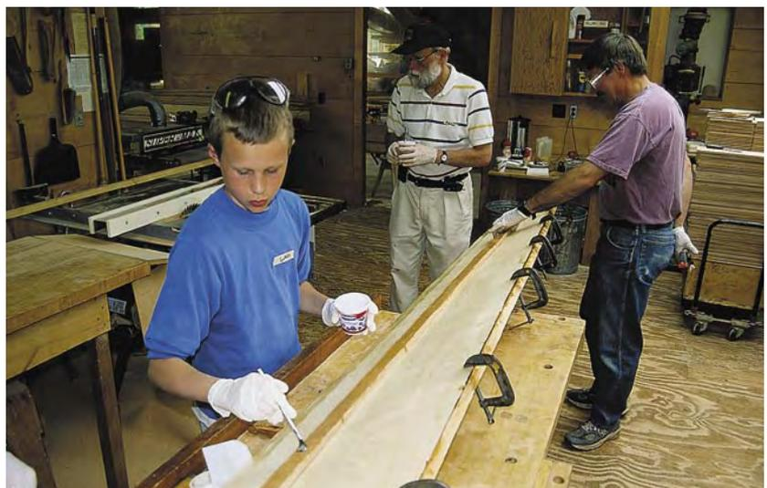
At the class, just as in your shop, boat building begins with assembling all the side plywood and connecting pieces during an intense three-hour session. While the epoxy remains wet the boat sides will be sprung into shape. Here Lars Hamre (left) and Jim Hott (right) spread epoxy on the gunwale that goes along the top edge of the side panel. The chine log is already clamped to the edge where the panel and bottom will meet. Lars came with his father, Merlin Hamre (middle).
