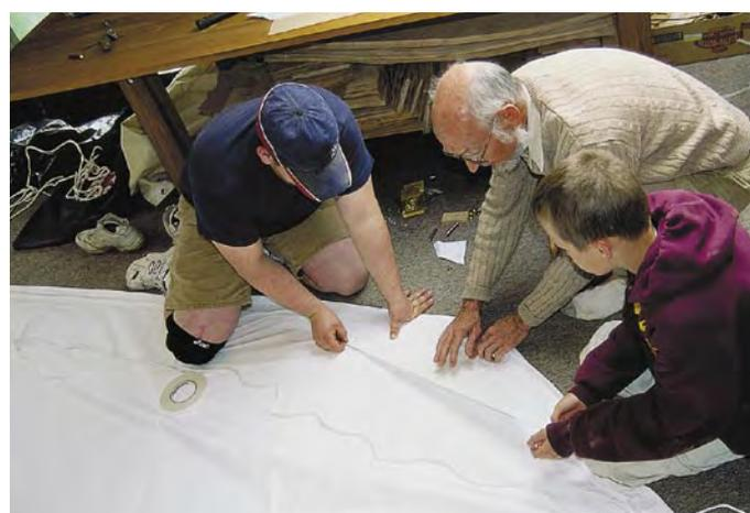
The sail is made from Tyvek in a cloth finish rather than the stiffer building wrap used in home construction. The cloth comes 10' wide, thus avoiding the need for any center seams. From left to right, my partner, Eric Pintar, I and Lars use seam tape to add reinforcements into the corners.
