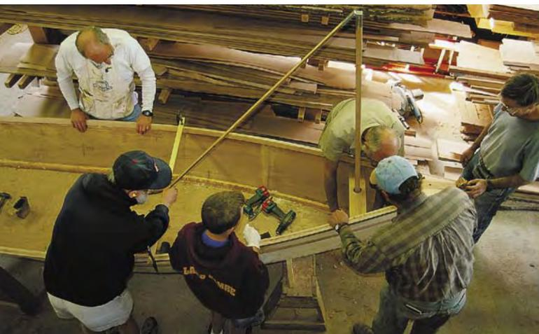
An important aspect of the set of the sail is the location of the mast and the angle at which the mast is held in the step. Here a simple jig is used to locate the mast step under the cross piece with the hole called the mast partner.
