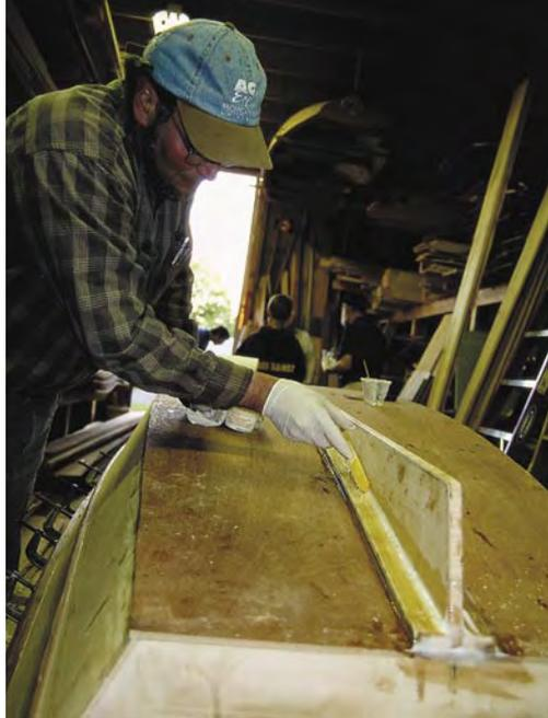
A key skill in using plywood for any boat more than 8' long is being able to scarf pieces to required length, as shown on page 88. The scarf joint is made by tapering the ends to be joined, thereby exposing wood fiber along their stronger orientation. The normal cut is a 1:8 to 1:12 ratio of thickness to length of the joint. In solid wood the joint strength will come close to that of a continuous piece.
