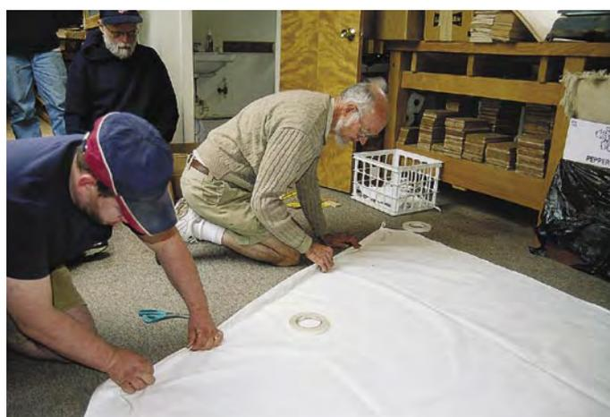
Pintar and I hem the sail all around using seam tape. A bolt rope and grommets will add strength to the hem. The corners can be stitched by hand or by a sewing machine.
