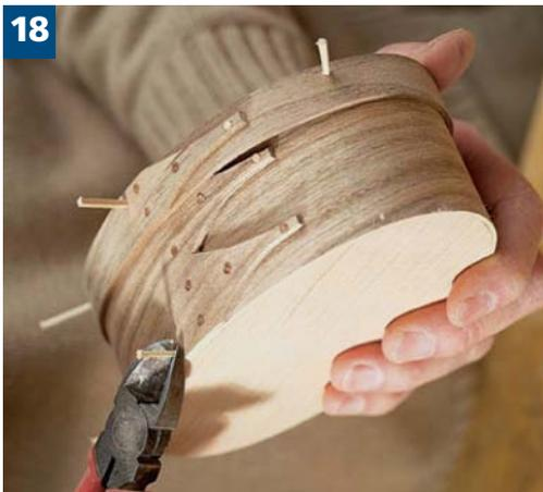
Wood pegs are made from cutting in half the box of World's Fair Brand toothpicks. The tapered end of these match the  $\frac{5}{64}$ " hole for a secure fit when tapped in place.
