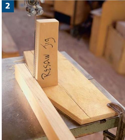
Resawing on the band saw can handle stock of 6" or more depending on the capacity of your machine. The resaw jig guides the cut. Clean up the board's sawn edge between each cut to give one smooth side. A drum sander gives a finished face to the sawn side. The blade shown is a 1/4" Timber Wolf four-teeth-per-inch band that's used for general work in my shop. Others prefer a silicon-carbide hook-tooth 1/2" or 3/4" blade.
