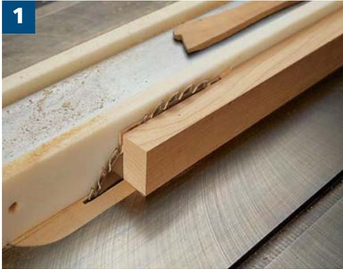
The table saw is my tool of choice for resawing bands up to 3" wide, although things slow down appreciably when nearing the capacity of the 10" blade. A sharp blade is a must. The zero-clearance wood insert shown here will prevent the thin wood from dropping through the table. When your setup is cutting effectively, there is little sanding required.
