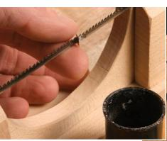
Place silver alloy in ribbon form between the two scarfed ends of the blade (above). Add flux to the joint using a small shop scrap (right).
