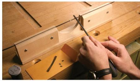
Align the two ends of the sawblade in your jig. Sight across the blade and use a screwdriver to tap the ends into position.
