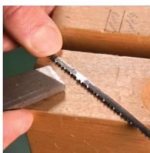
**The final step** is to file off the burrs at the joint and remove the glass-like residue left by the flux.
