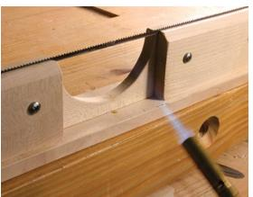
**Remove the brittleness** from the band by heating the joint using successively less and less heat. Back up the torch on each pass.
