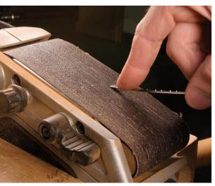
Cut your band 1/4" longer to allow for the overlap at the joint. Here we're using a belt sander to bevel one end of the band to create the scarf joint.
