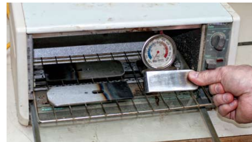
TEMPERING IN OVEN and holding at 400° F for 20 minutes and cooling slowly will restore needed toughness. Polish and sharpen cutter, but leave reverse side rough to help hold securely in plane.
