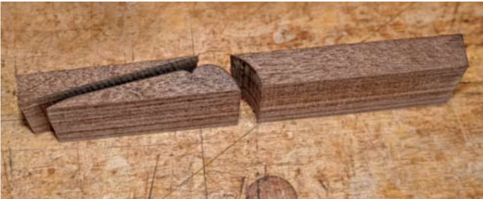
CUT WEDGE from \frac{1}{2} " x 1\frac{1}{2} " stock. A 9^\circ wedge is cut from end corner back 3". Sand micro bevel on lower end. Notch top. Sand true.
