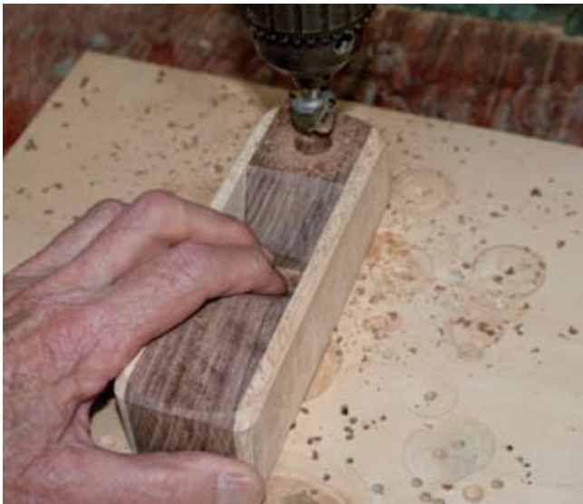
DIMPLE FORE BLOCK FOR FINGER HOLD using a router core bit chucked into the drill press. Note edge chamfering and corners rounded.
