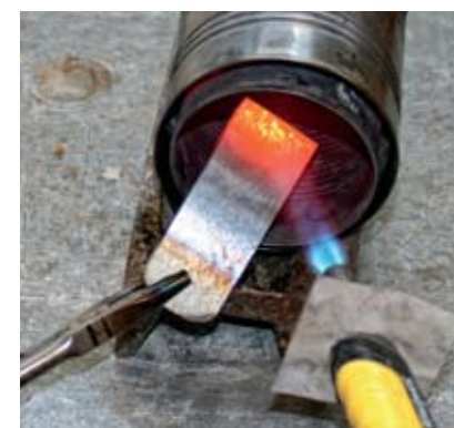
TOOL STEEL IS HEATED to cherry red using a torch and tin can "furnace" to focus heat. Quench in oil to make it hard and brittle. CAUTION: Tin can gets hot. Keep away from flammable surfaces.
