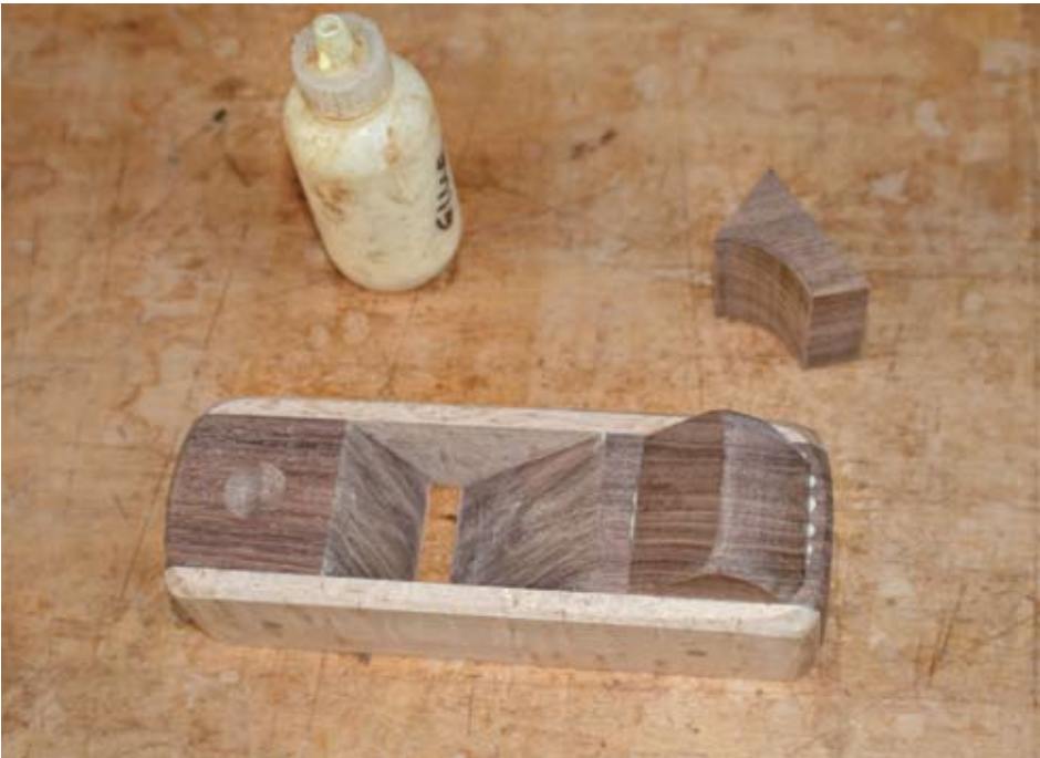
HEEL BLOCK IS CUT FROM THROAT SCRAP. Here you see the remainder behind it on the bench. Round over edges. Leave \frac{1}{4} " space between bedding angle and heel block for hammer tapping the blade.
