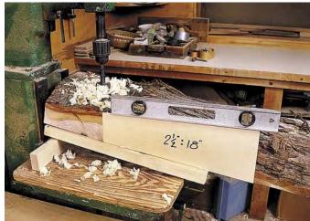
To achieve the desired leg splay, use a level on top of a board cut to the ratio of  $2^{1}/2$ " to 18". This is the angle both end-to-end and side-to-side. The heavy slab rests on wood blocks to steady the drilling with a  $1^{3}/4$ " Forstner bit in the drill press.
