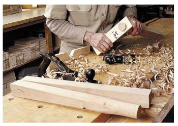
If you don't own a rounder plane, you can use a block plane to form the tenon. Whichever method you choose, use a hole gauge to check the tenon's size.
