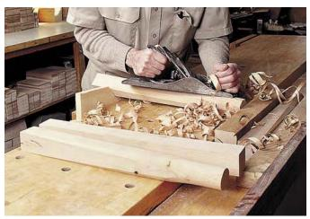
Prepare the legs using a V-notched board and a stop block. Plane the 2" x 20" squares so the bottom remains square and the top end is octagonal.
