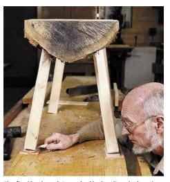
The final leg length is marked by leveling the bench (note the use of wood scrap under each shorter leg) and marking with a scribe. Cut along the lines and plane all sharp edges as the final step.
