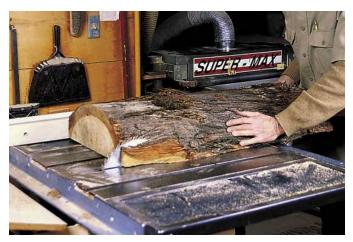
Trimming the top to size can involve a variety of tools: table saw, circular saw or chain saw. Leave an edge about  $1^{1/2}$ " wide.
