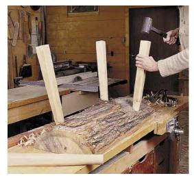
Hammer the legs into place. With this version of the garden bench with stopped holes, no glue or wedges are necessary, as the legs, being drier than the slab top, will hold tight as the top dries.
