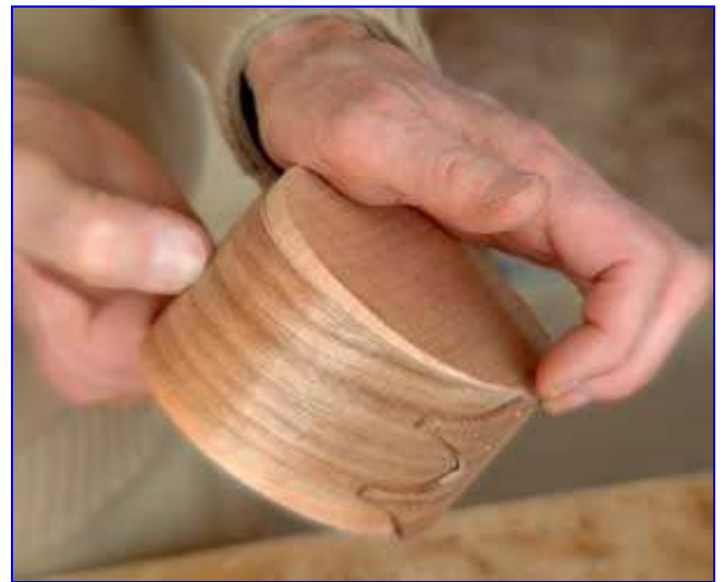
Photo 15. Inserting Oval Board
