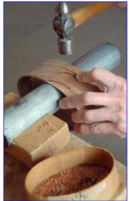
Photo 9. Clinching Lap with Copper Tacks
