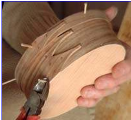
Photo 18. Inserting Wood Pegs
