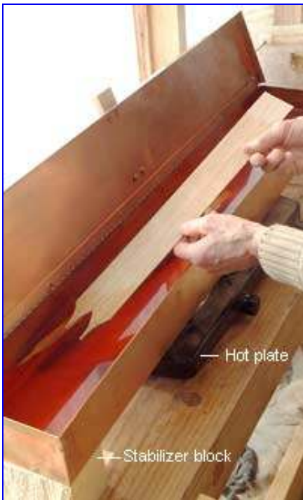
Photo 7: Hot Water Tray
