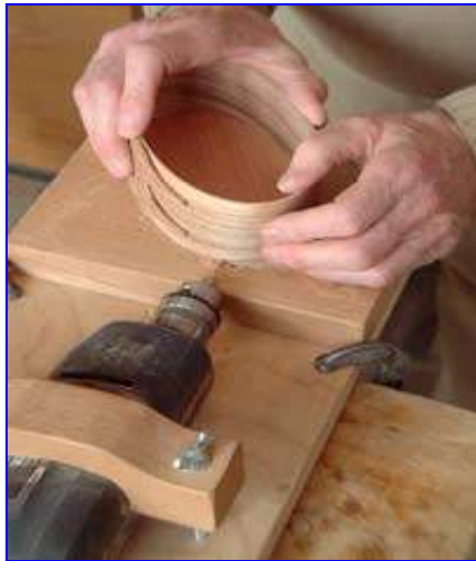
Photo 16. Drilling Perimeter for Wood Pegs
