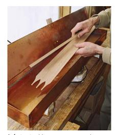
In hot water. My copper water tray sits on a hot plate, with wood blocks under each end for stability. A full boil is not necessary; 180° F will soften the lignin sufficiently for bending in about 10-20 minutes.
