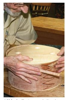
Add the rim. The rim gets tucked into the curve of the top finger and ends with a 4" lap that will project about 1" beyond the fingers. After bending the rim in place, remove the top shaper and hold the rim in place (a spring clamp might help) as you drill 1/16"-diameter pilot holes every 3" for the escutcheon pins (with three holes 2" apart at the lap).
