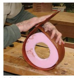
**Bending.** Remove the band from the hot water and bend it around the form. You're aiming only for the approximate shape, so don't fuss with wrapping it tightly.
