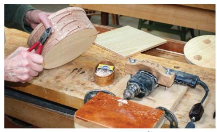
**Secure the bottom.** I use toothpicks to secure the bottom, drilling  $\frac{5}{64}$ " pilot holes every 2"-3" around the box, centered in the thickness of the bottom. After tapping the toothpicks in place, I use side cutters to snip them off, then sand smooth.
