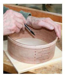
Mark a circle. Once the band and rim are thoroughly dry, the box will hold its round shape. So you can use it as the template for marking the bottom board.
