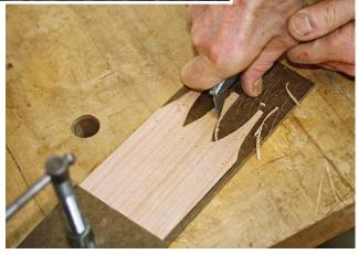
Carving. I use a utility knife with a fixed, heavy-duty blade to trim the fingers to final shape, and to cut a slight bevel on the edges.
