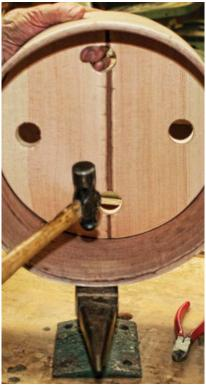
**Snip, file & peen.** Snip the end of the escutcheon pins as close as possible, then file them close to flush before peening.
