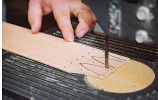
Fingers. Use a band saw to remove the waste and cut to rough dimensions. Now drill holes in the marked locations for the copper tacks.
