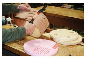
The right size. Remove the form, then match the feathered end to the penciled circumference mark. Use a scrap of wood and spring clamps to hold the fingers in place.
