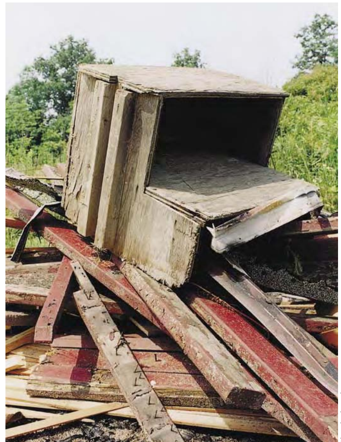
Here is the old stool after a life of usefulness, now on the burn pile to be returned to basic elements of the universe and to be recombined into a new generation of materials. Note the badly worn corners where the plywood feet gave out. The attachment of the hardwood "shoes" as I describe in the article will extend the life of your stool.
