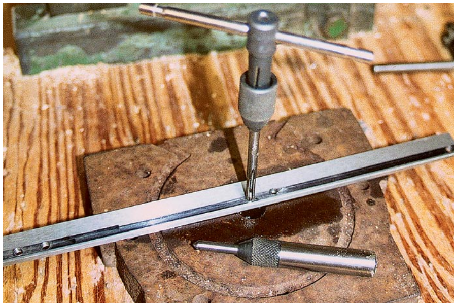
Tap first. An 18" length of O1 tool steel \frac{1}{8} " x \frac{5}{8} " will make four spokeshave blades. Black magic marker is used to highlight layout lines to locate holes for 10-32 threaded rod posts. Here a tap and tap wrench are used in a setup on the drill press using a spring-loaded center (taken out of the drill chuck for viewing purposes) to keep the tap straight while threading.
