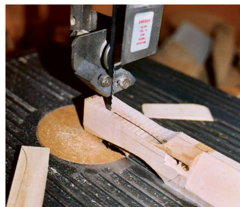
Rough out the handles. The handles are roughed out on the band saw or with a coping saw. The shape is individual. I use the roller end of a belt sander for smoothing and chamfering the edges, preferring handles that have some "edge" rather than smoothly rounded ones.
