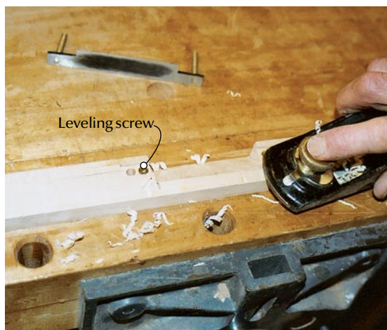
Bevel blade approach. The approach to the blade is beveled to allow for the curvature of the wood to be shaved. A general angle of 8° is planed here using a block plane. With that, the cutting part of the spokeshave is done.
