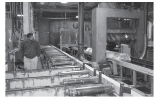
Here come the flitch. Having been fished out of the hot water vat, they are cleaned all over to remove the resulting black layer: sides milled, ends trimmed, and back planed flat which is happening here.
