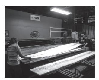
$20\,$  The speed of the conveyor and the temperature of the blown air result in the final moisture in the wood. Bending stock wants to be dry enough not to mold (under 20° MC) and not as dry as standard veneer destined for panel facing (6° MC).
