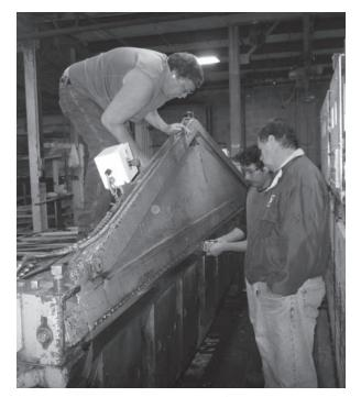
$10^{\circ}$  Correct adjustment is critical for producing quality slicing. At left you see the mill operator wrenching the bolts to adjust the lead and gap that exert the necessary pressure for a smooth, tight veneer. The man in the center holds a gauge while the plant manager looks on.
