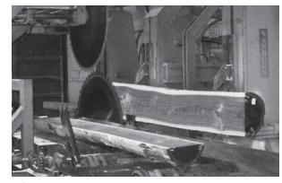
Cutting down the center creates two halves called flitches. The alternative method of veneering is to rotary cut in the round. Only by flitch cutting will the grain pattern of sawn lumber be preserved. It also results in the best bending stock.
