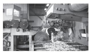
3 Debarking is the first stop on the journey through the mill. This will not only remove unwanted bark, but dirt and grit that dulls saw and knife.
