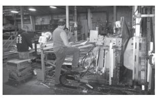
Viewed from the side are parts of the Capital slicing machine, patented in 1905. From right to left: the vacuum and dogging flitch holder which travels up and down; the flitch; the knife and nose bar; the carriage which advances with each slice; the conveyor with veneer slices; and catchers stacking veneer.
