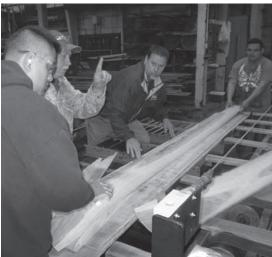
$16\,$  "Stop the mill." The final adjustments will happen as thickness and surface are checked.
