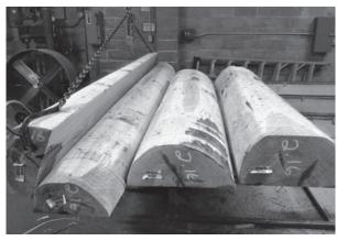
$12^{\,\,\,}$  Clean as plucked chicken, the flitch await mounting on the mill. The one on the left is being hoisted with chain and hooks.
