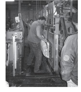
$13^{(right)}$  The flitch moves onto the mill where it is mounted with a combination of holding dogs and suction. The dogs will retract after the bulk of the flitch is sliced, leaving the remainder held by vacuum alone. The mill can leave as little as  $^{1}/4$ " of wood unsliced.
