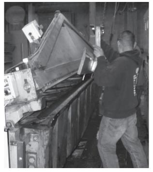
9 The knife is being installed. It will take about two hours from this point until all six logs, twelve flitch, are sliced.
