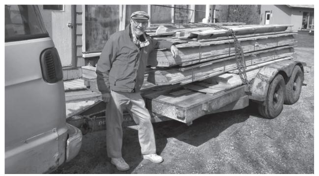
Home again and parked in the drive outside the shop. All six cherry logs are now twelve crates of thick bending stock veneer. The two thicknesses of  $^{1}/_{10}$ " and  $^{1}/_{12}$ " will be graded, cut in stacks of 10 into dimension, and drum sanded where necessary for final band stock.
